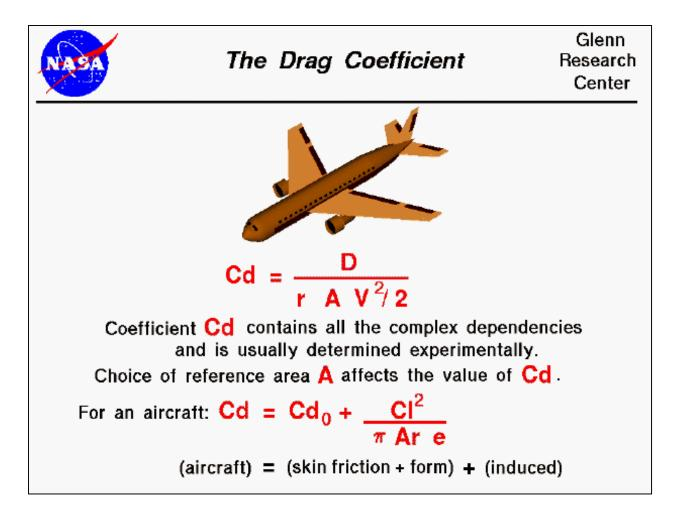
The drag coefficient is a number that aerodynamicists use to model all of the complex dependencies of drag on shape, inclination, and some flow conditions. This equation is simply a rearrangement of the drag equation where we solve for the drag coefficient in terms of the other variables. The drag coefficient (Cd) is equal to the drag (D) divided by the quantity: density (r) times half the velocity (V) squared times the reference area (A).
