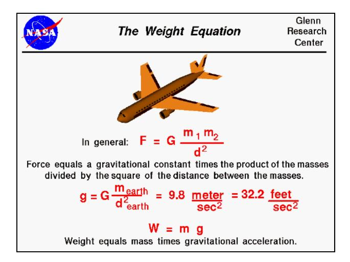
Weight is the force generated by the gravitational attraction of the earth on an airplane or model rocket. Weight is fundamentally different from the aerodynamic forces, lift and drag. Aerodynamic forces are mechanical forces and the vehicle has to be in physical contact with the air which generates the force. The gravitational force is a field force; the source of the force does not have to be in physical contact with the object (the airplane or rocket).
