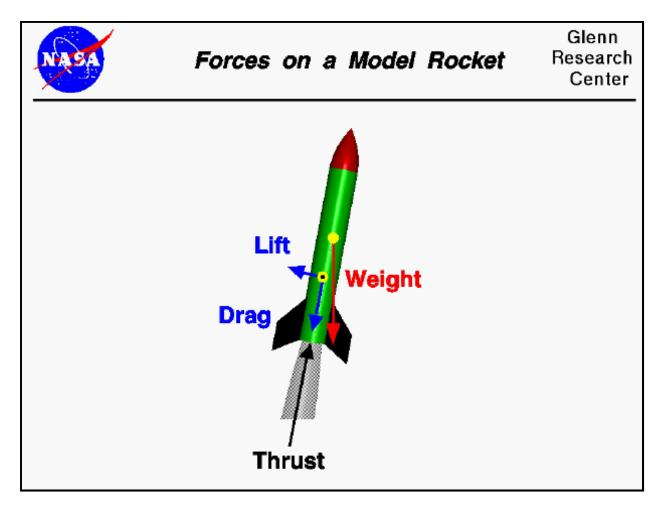
Flying model rockets is a relatively inexpensive way for students to learn the basics of aerodynamic forces and the response of vehicles to external forces. Like an aircraft, a model rocket is subjected to the forces of weight, thrust, drag, and lift. There are, however, some important differences in the actions of these forces on a model rocket as opposed to a powered aircraft or a glider:
