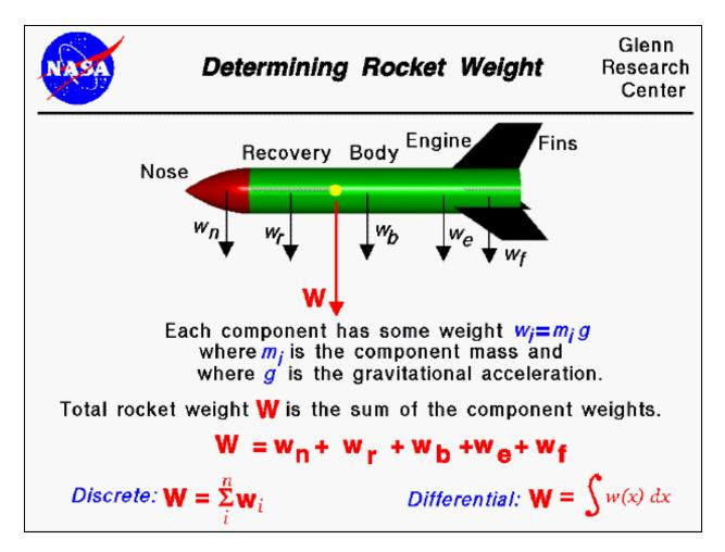
Weight is the force generated by the gravitational attraction of the earth on the model rocket. The mass (and weight) is actually distributed throughout the rocket and for some problems it is important to know the distribution. But for rocket trajectory and stability, we only need to be concerned with the total weight and the location of the center of gravity. The center of gravity is the average location of the mass of the rocket.
