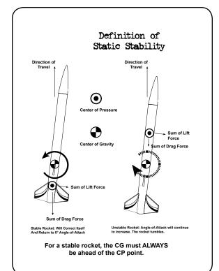
**Purpose:** To illustrate the definition of stability. If the CP is forward of the CG, the angle-of-attack will increase when a force pulls on the CP point.
