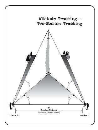
**Purpose:** To show the geometry of tracking a model rocket using two trackers that are each taking elevation and azimuth angle readings from a theodolite.
