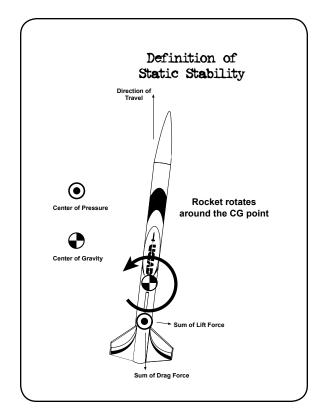
**Purpose:** To show the students that any object will rotate around its own CG point. A torque is produced by the aerodynamic forces acting at the CP point. This is what causes the rotation around the CG point.
