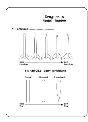
**Purpose:** To illustrate the first component of drag on a rocket: Form Drag.
