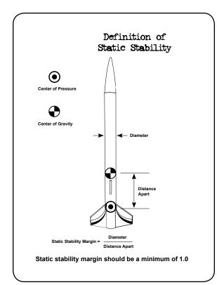
**Purpose:** To illustrate a minimum safety requirement for model rockets.
