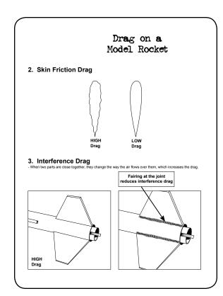
**Purpose:** To illustrate the next two components of drag on a rocket: Skin Friction and Interference Drag. The surface texture of the rocket, how smooth it is, determines the amount of skin friction drag the rocket will have. Smoothing airflow in tight corners will help reduce interference drag.
