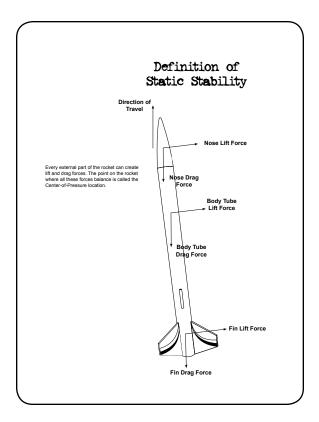
**Purpose:** To show that each component (not just the fins) creates both lift and drag when flying at an angle-of-attack. The fins produce the most forces, but the other parts contribute as well.
